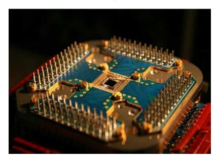
Figure 20. First commercially available quantum processor (D-Wave Systems)
